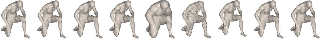
Figure 6. SHREC benchmark dataset. The transformations are (from left to right): isometry, holes, micro holes, scale, local scale, noise, shotnoise, topology and sampling.
